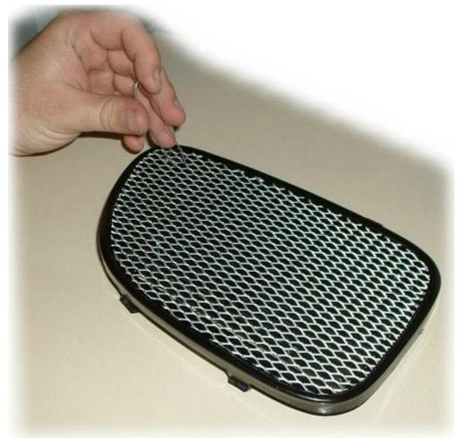
3. Take about 6-7" of the wire and bend it in a V shape and run it through two adjacent diamonds that overlay a stock horizontal bar. Ties can be used instead of the wire if desired.
