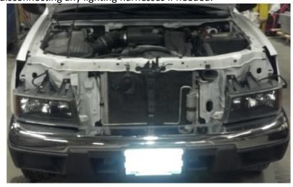
3. Place a clip through the mesh, near the outside perimeter of the grill. For best results, you should start from the center and work your way to the sides. You may need to straighten or bend the clip to manipulate it a way that will make it feed through properly.
