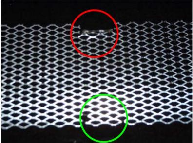
b. Attach the clips. There are three sections on the bottom of the grill where three clips need to be installed.Each of the three sections has two diamonds and cut next to them like the green circled area.c. Hook the two prongs on the clip around the diamonds and tighten down like so.
