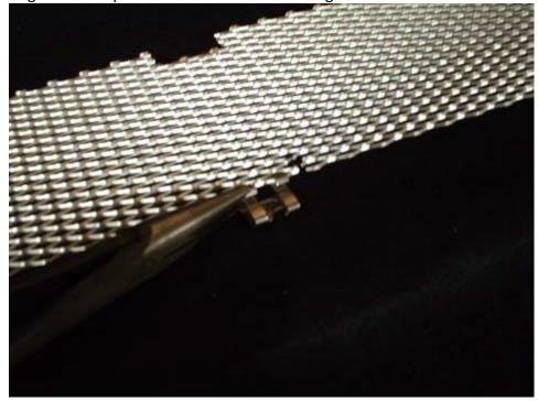
d. Then tighten down the back part of the clip. If you do no tighten down enough, the clip will not hold well on the bumper. If you tighten down too much, it may be difficult to install.
