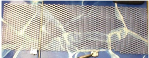
4. Now turn the grill around and tighten down the clamping part of the clip to the desired tension. Just take your pliers and close the gap down as far as you want. If you don't tighten them down enough, they will not hold and if you tighten them too much it will be hard to install.
